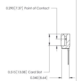
ACAD REFERENCE NO. 746-ENG MASTER 746 Series Ultra-Mate Card Edge Connector - Press Fit DRAWN: J.LEE DATE: AUG 20/09 Part Number: 746-007-553-101 CHECKED: DATE: **EDAC INC** SCALE: SHEET 1 OF 1 THESE DRAWINGS AND SPECIFICATIONS ARE THE PROPERTY OF EDAC INC.,AND TORONTO, ONTARIO SHALL NOT BE REPRODUCED, OR COPIED DRAWING NUMBER CANADA OR USED AS THE BASIS FOR THE 746-ENG MASTER MANUFACTURE OR SALE OF APPARATUS YOUR CONNECTION TO QUALITY & SERVICE WITHOUT WRITTEN PERMISSION.
