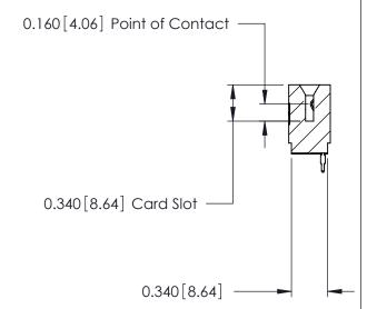
ACAD REFERENCE NO. 746-ENG MASTER 746 Series Ultra-Mate Card Edge Connector - Press Fit DRAWN: J.LEE DATE: AUG 20/09 Part Number: 746-008-525-501 CHECKED: DATE: SCALE: SHEET 1 OF 1 **EDAC INC** THESE DRAWINGS AND SPECIFICATIONS ARE THE PROPERTY OF EDAC INC.,AND TORONTO, ONTARIO SHALL NOT BE REPRODUCED, OR COPIED DRAWING NUMBER CANADA OR USED AS THE BASIS FOR THE 746-ENG MASTER MANUFACTURE OR SALE OF APPARATUS YOUR CONNECTION TO QUALITY & SERVICE WITHOUT WRITTEN PERMISSION.
