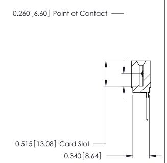
ACAD REFERENCE NO. 746-ENG MASTER 746 Series Ultra-Mate Card Edge Connector - Press Fit DRAWN: J.LEE DATE: AUG 20/09 Part Number: 746-017-540-101 CHECKED: DATE: **EDAC INC** SCALE: SHEET 1 OF 1 THESE DRAWINGS AND SPECIFICATIONS ARE THE PROPERTY OF EDAC INC.,AND TORONTO, ONTARIO SHALL NOT BE REPRODUCED, OR COPIED DRAWING NUMBER **ISSUE** CANADA OR USED AS THE BASIS FOR THE 746-ENG MASTER MANUFACTURE OR SALE OF APPARATUS YOUR CONNECTION TO QUALITY & SERVICE WITHOUT WRITTEN PERMISSION.
