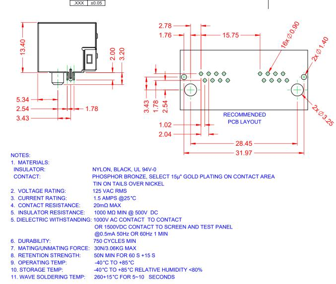
MATES WITH MODULAR PLUG CONFORMING TO FCC PART 68, SUBPART F.
