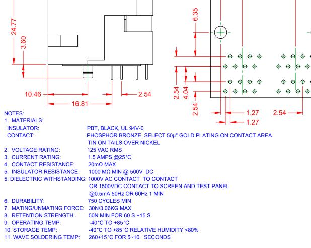
MATES WITH MODULAR PLUG CONFORMING TO FCC PART 68, SUBPART F.
